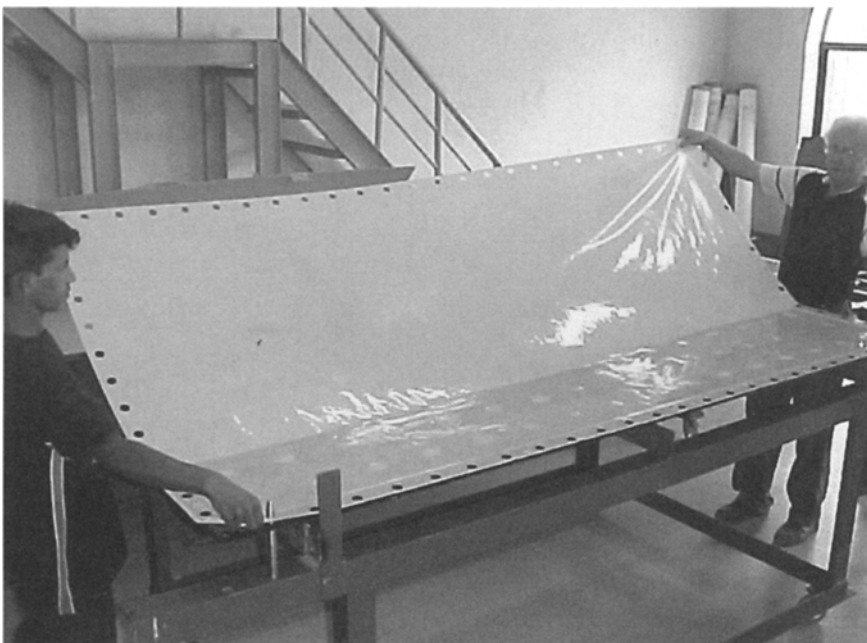
FIGURE 13.6. Fitting membrane to a large bipolar electrode (with permission of INEOS Chlor Limited).
