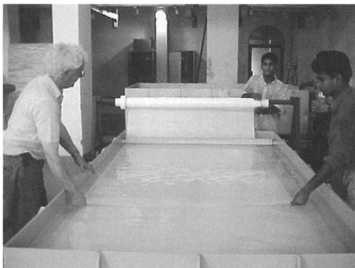
FIGURE 13.2. Unrolling of membranes into bath (with permission of INEOS Chlor Limited).
