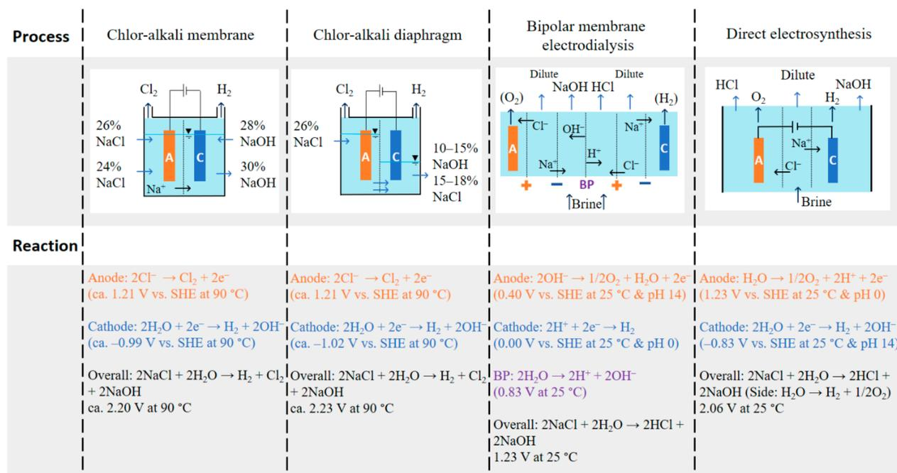
**Figure 1.** Schematic diagram of a chlor-alkali membrane, a chlor-alkali diaphragm, a bipolar membrane electrodiolysis, and a direct electrosynthesis process. The half-reactions and energy requirements are given (sources: chlor-alkali processes,<sup>1</sup> bipolar membrane electrodiolysis,<sup>2</sup> direct electrosynthesis<sup>3</sup>). Key: A, anode; C, cathode; BP, bipolar membrane; NaOH, sodium hydroxide; HCl, hydrochloric acid.
